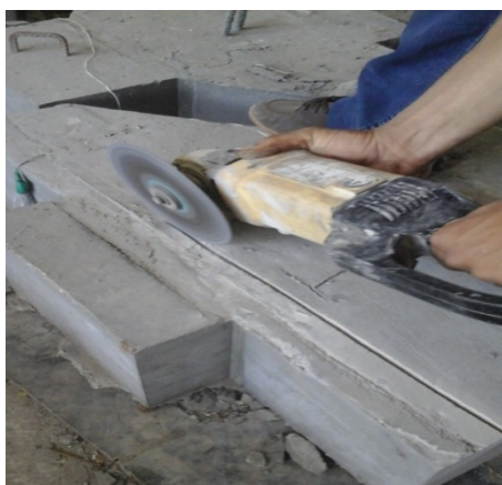
Plate 2 : grooves in concrete corbel in each face
